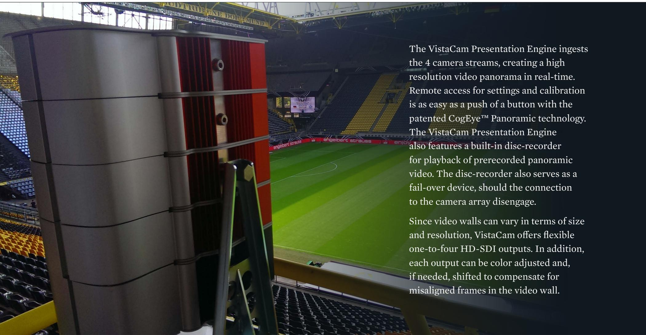
The VistaCam Presentation Engine ingests the 4 camera streams, creating a high resolution video panorama in real-time. Remote access for settings and calibration is as easy as a push of a button with the patented CogEye™ Panoramic technology. The VistaCam Presentation Engine also features a built-in disc-recorder for playback of prerecorded panoramic video. The disc-recorder also serves as a fail-over device, should the connection to the camera array disengage.
